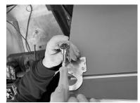
16. Adjust the doors using the bottom hinge that moves front to back and the hinge that moves horizontally from left to right so that it closes tightly. Once the door is properly positioned, screw in the bottom hinge and the center hinge. You can now put the refrigerator back upright and make sure the doors close properly.
