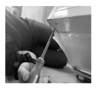
9. Locate the hinge support bag included in the refrigerator. Unscrew the refrigerator and freezer door hinge supports from the refrigerator door and freezer door. Install new hinge brackets on the left-hand side of both doors.
