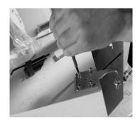
13. Remove the plastic cap on the left-hand side of the top of the refrigerator and install it on the right-hand side to cover the holes in the old hinge.
