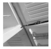
5. Unscrew the center hinge using the 5/32 Allen Key and remove the bottom door by sliding it upwards
