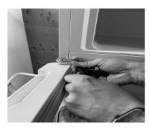
NB: Do not screw all the way in, as these screws are used to adjust the doors.
