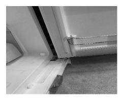
6. Remove the lugs and remove the hinge under the refrigerator using the ratchet wrench and 8mm socket or Philipps screwdriver no.2.
